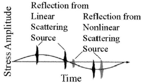
Figure 13. Amplitude modulation of HF 'probe' pulse by LF 'pump' wave (after Kazakov et al. [6]).
