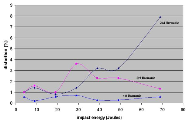
Figure 8. Detection of impact damage in CFRP plate by the single-frequency harmonic method (after Armitage [5]).
