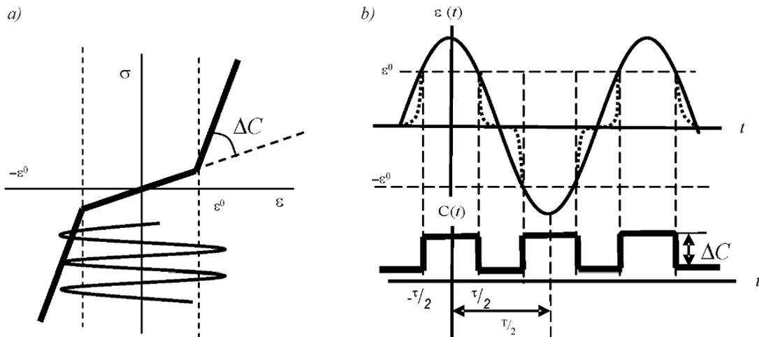
Figure 4. a) Non-linear stress-strain curve and (b) waveform distortion (upper) and stiffness modulation (lower) for stick-slip friction-based non-linearity (after Solodov [3]).
