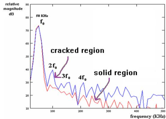
Figure 7. Detection of compressive damage in concrete by the single-frequency harmonic method (after Armitage [5]).
