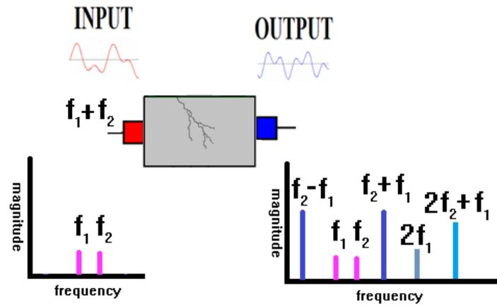
Figure 9. Dual-frequency intermodulation (after Armitage [5]).
