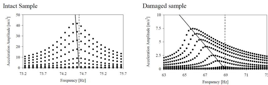
Figure 16. Measured resonance curves at varying input (strain) levels (after Van Den Abeele [8]).
