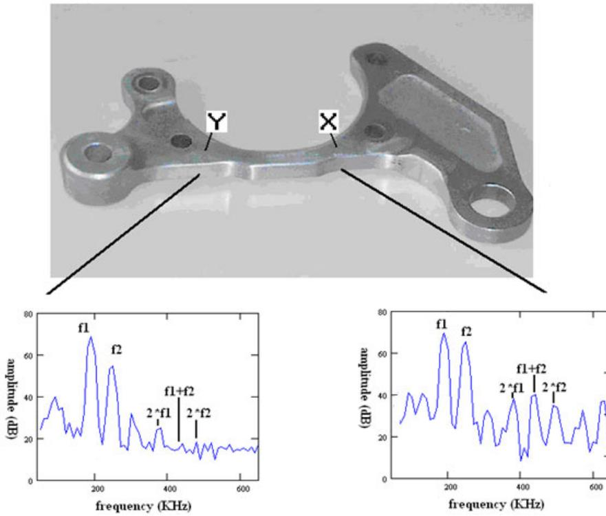
Figure 11. Dual-frequency (184kHz and 240kHz) intermodulation detection of early-stage failure in a safety-critical aircraft component (after Armitage [5]). After 20,000 stress cycles, a defect is indicated at point X. The component failed at this point after 120,000 cycles.
