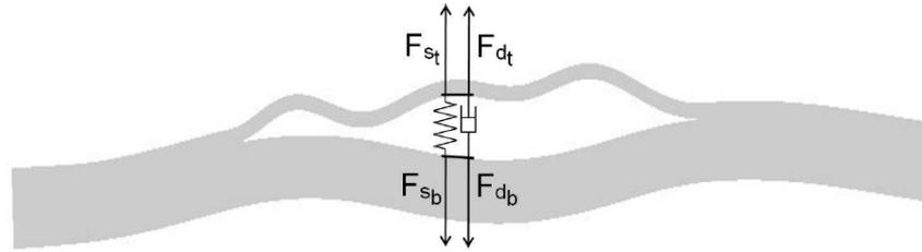
Figure 3. Spring and damper elements implementing a simple model of a delamination (after Delrue [4]).
