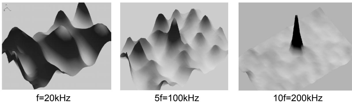
Figure 6. Resolution of defects using high-order harmonics (after Solodov [3]).
