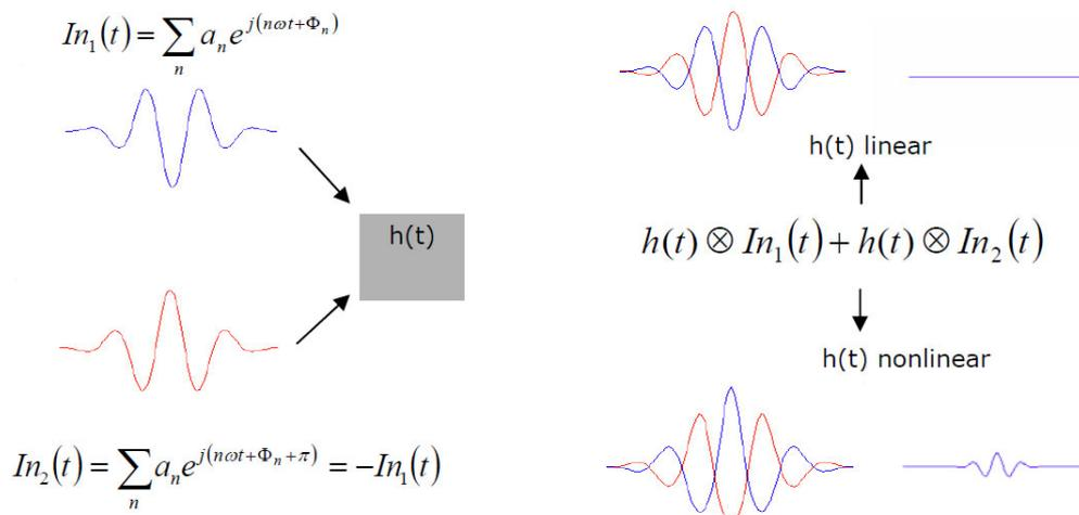
Figure 14. The principle of the pulse inversion method (after Mattei [7]).
