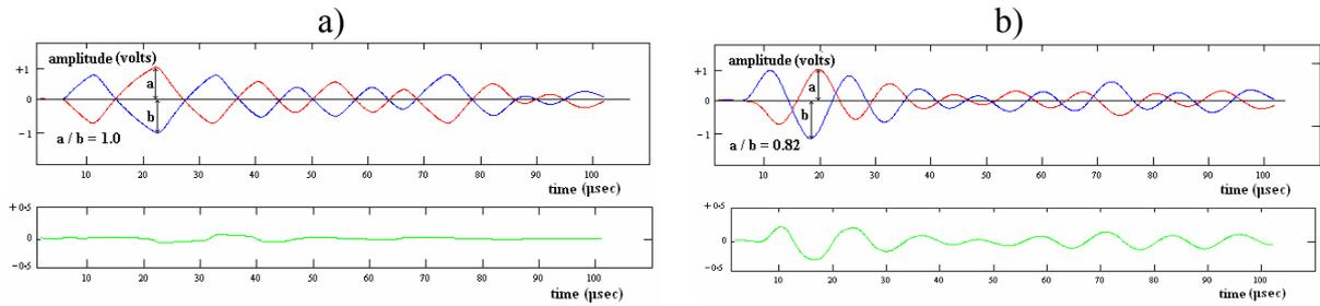
Figure 15. Response of carbon fibre laminate to positive pulse (blue) and negative pulse (red) and the summation of these responses (green): a) intact panel; (b) damaged panel (after Armitage [5]).
