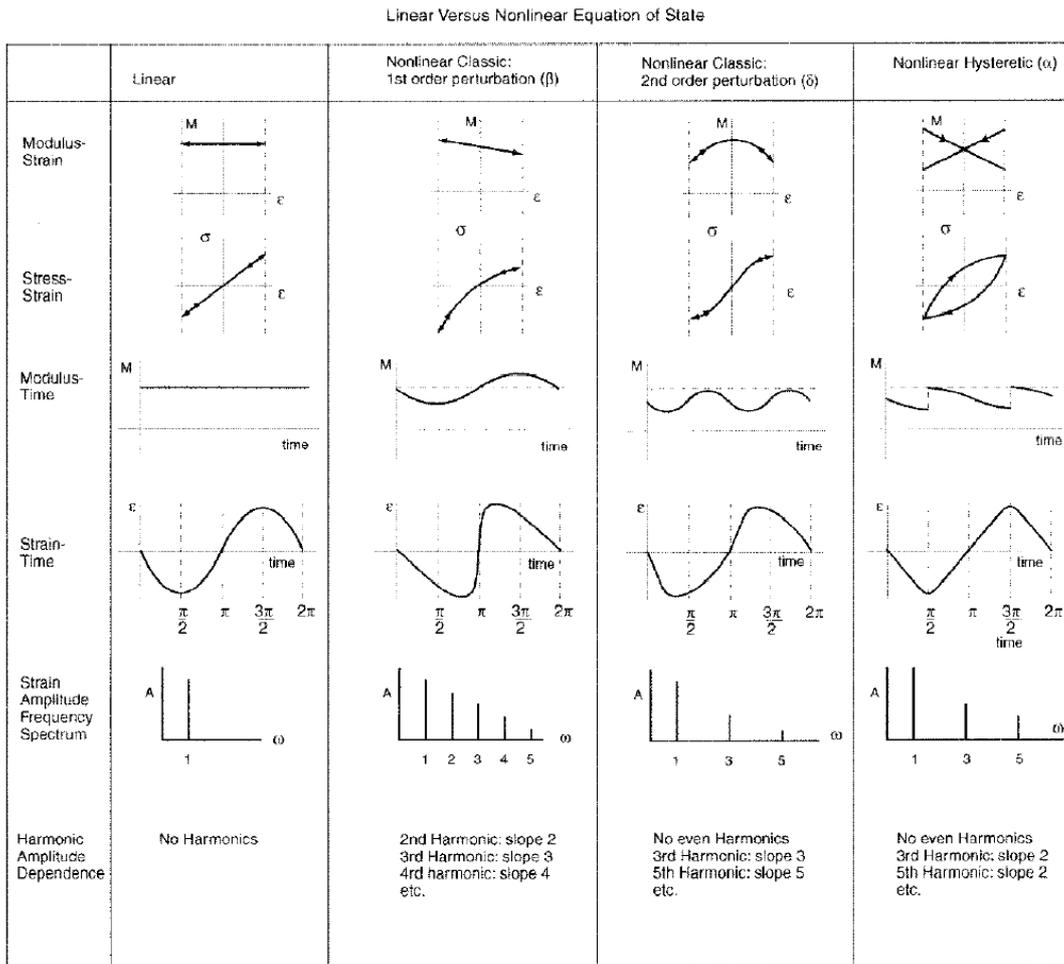
Figure 5. The various non-linear manifestations of structural defects (after Van den Abeele [2]).
