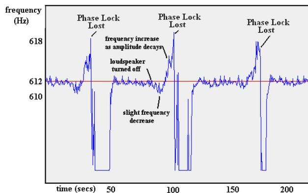
Figure 17. Real-time measurement of resonance frequency drift in a flawed structure using a phase-locked loop (after Armitage [5]).
