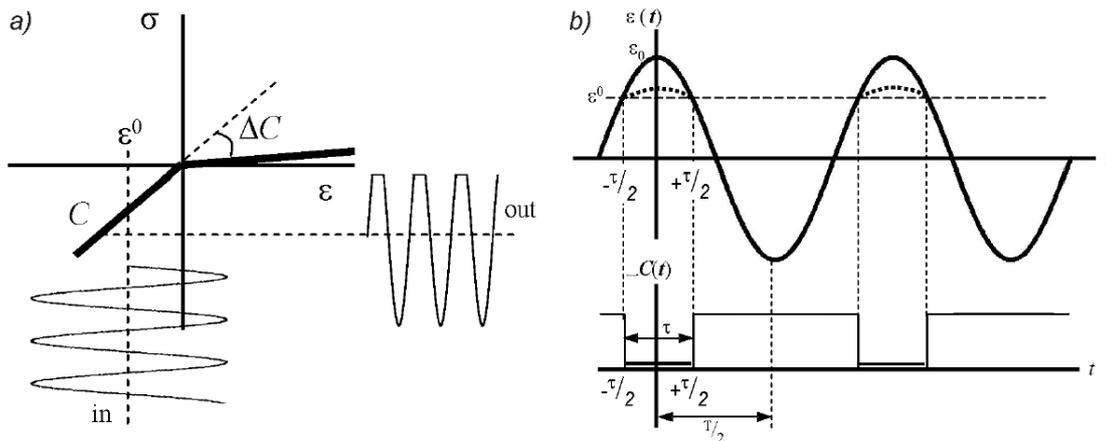
Figure 1. a) Non-linear stress-strain curve and (b) waveform distortion (upper) and stiffness modulation (lower) for clapping non-linearity (after Solodov [3]).
