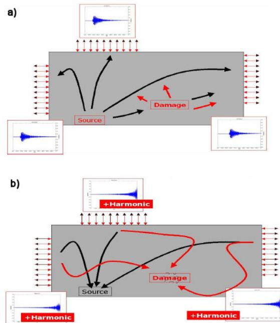
Figure 18. a) In a structure containing a non-linear defect, harmonics will be generated at the damage site. b) Transmitting back the time-reversed signals will result in two concentrations of energy – one at the original source site and the other (harmonics) at the defect (after Armitage [5]).
