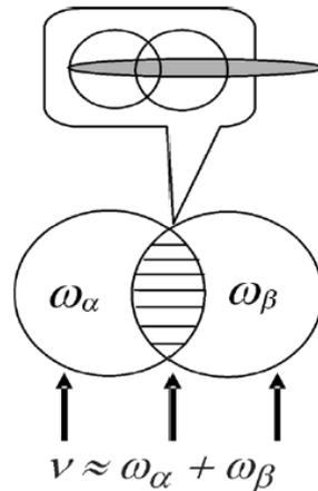
Figure 2. Representation of a crack as a pair of coupled oscillators. If the frequency of the excitation is  $v \approx \omega_\alpha + \omega_\beta$ , the difference frequency components  $v - \omega_\alpha \approx \omega_\beta$  and  $v - \omega_\beta \approx \omega_\alpha$  provide cross excitation of the coupled oscillators. (after Solodov [3]).
