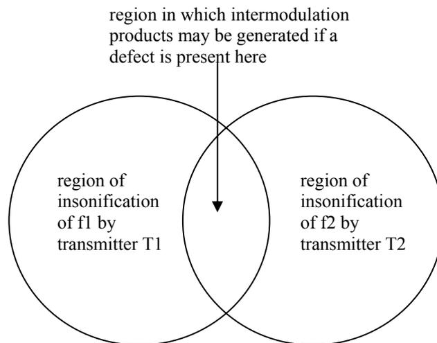
Figure 12. The ability of dual-frequency intermodulation to locate defects through overlapping regions of insonification.
