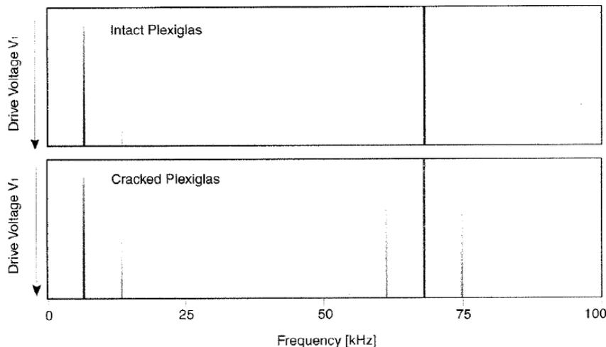
Figure 10. Dual-frequency (7kHz and 70kHz) intermodulation detection of damage in Plexiglas (after Van Den Abeele[2]).
