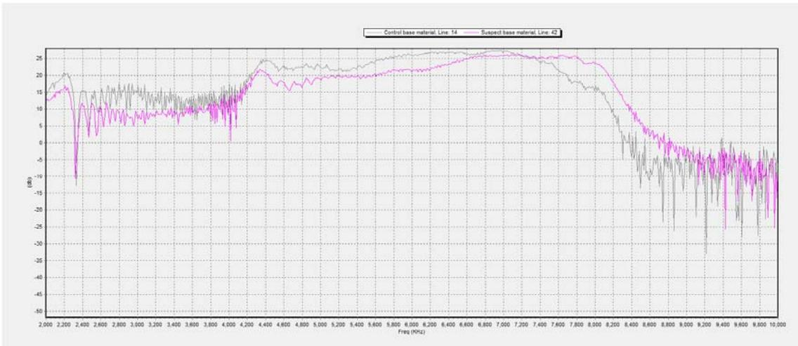
Figure 4 - Inspection of spectra taken from centre of base material scans on control and suspect samples
