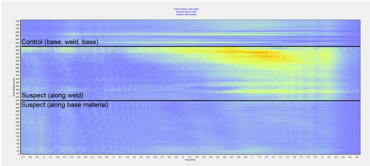
*Figure 9 - Combined view of suspect base material, suspect weld and control scanned across weld*
