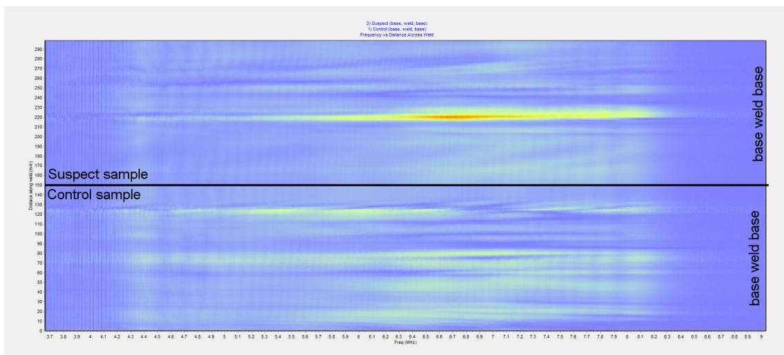
Figure 8 - Scan across the weld of the control and suspect samples
