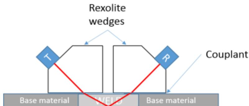
Figure 1 - Pitch-catch head assembly schematic. T is the transmitter, R is the receiver
